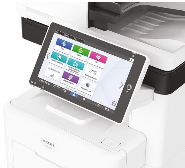
The versatile 4-in-1 MFP is equipped with a Single Pass Document Feeder (SPDF). To save time, double sided originals are scanned in a single pass and can be forwarded to email or uploaded directly to Cloud-share services, such as DropBox™ and Sharepoint™. The Smart Operation Panel also supports the use of enterprise workflow solutions, including Ricoh's Streamline NX. And, with Near Field Communication (NFC), secure authentication is as easy as tap and go.
